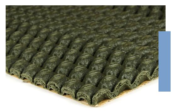
Specifications Floor Usage: Carpet Installation Method: Stretch Fit Construction: Sponge Rubber Thickness: 8.9 mm Square Weight: 3017 g/m<sup>2</sup> Roll Area: 15.07 m<sup>2</sup> End Use Classification GD/U General Use & Contract No Objectionable Odour Odour: French VOC Emission Regs: A+ Anti-Microbial & Mildew: Pass 35 dB Impact Sound Reduction: Recyclable: 100% Indoor Air Quality: Green Label Plus Certified
